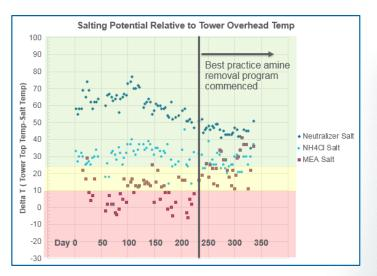
Figure 2: Field amine-chloride salting potential, using the PAT
