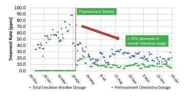
In another crude unit at the same refinery, pretreatment chemistry - asphaltene stabilizer - was injected into the raw crude and significantly reduced fouling in all hot pre-heat trains.
