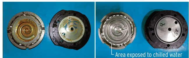
Mold inspection with TRAC 200 chemistry (L) and five months after (R) conversion to TRAC 2599. Source: Ecolab technical trial
